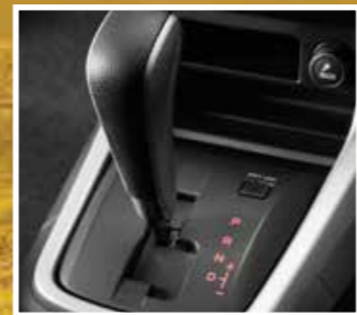
Fuel efficient sequential shift 5-speed automatic transmission
