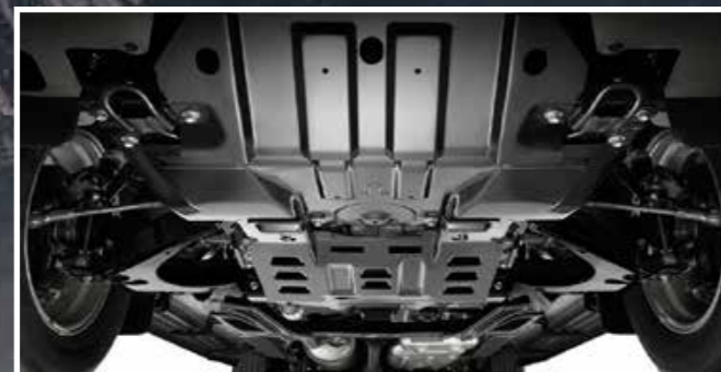
Steel underbody guards on sump and transfer case
