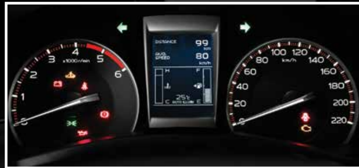
Electroluminescent instrument display gives clear vision to the driver
