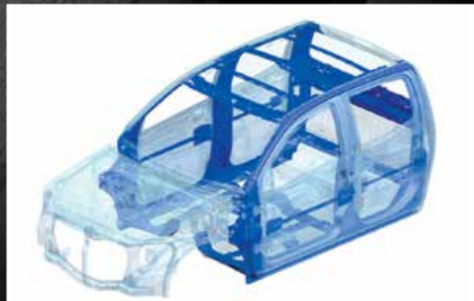
The cabin is constructed from high tensile tailor blank welded steel for unyielding strength and rigidity of the passenger safety cell
