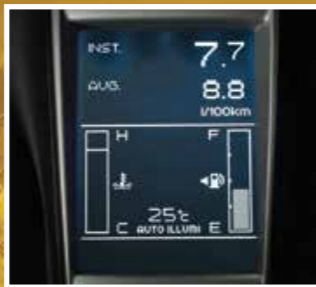
Multi Information Display of instant and average fuel consumption
