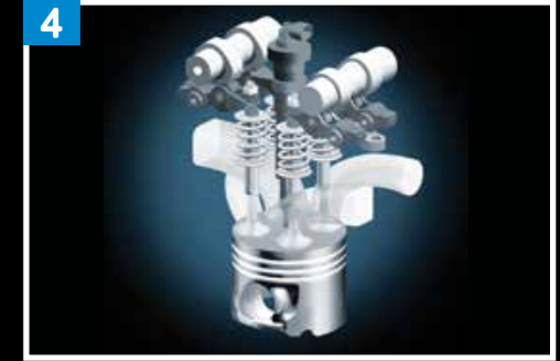
4 Sophisticated engine head; cam-to-valve roller bearings and variable swirl action gas flow
