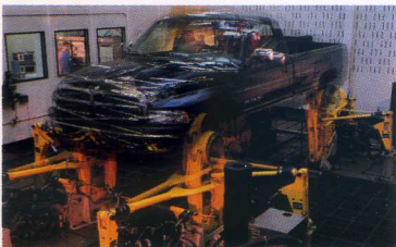
◆ Laboratory isolation testing on the suspension “Shaker” (Road Test Simulator) uses computer re-creations of the nation’s roughest roads to punish vehicles far longer and more severely than any real-world driver. Testing 18 days on the Shaker equals a 16-week, 20,000-mile endurance run.
