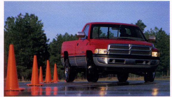
◆ The RAM’s suspension geometry and weight distribution include a low roll center to reduce side-to-side body roll during hard cornering.
