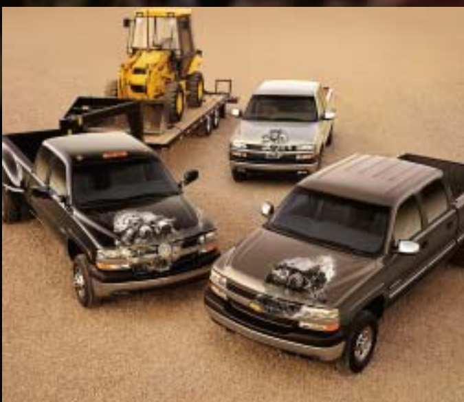
POWER. A strong Vortec engine is standard in every Chevy Silverado, including the 300-horsepower Vortec 6000 V8 SFI engine in 1500HD, 2500, 2500HD and 3500 models. Page 6.
